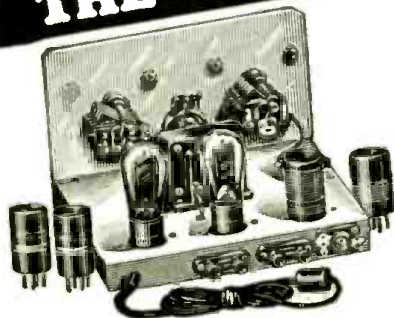
Rear View of Battery 2-Tube Set
