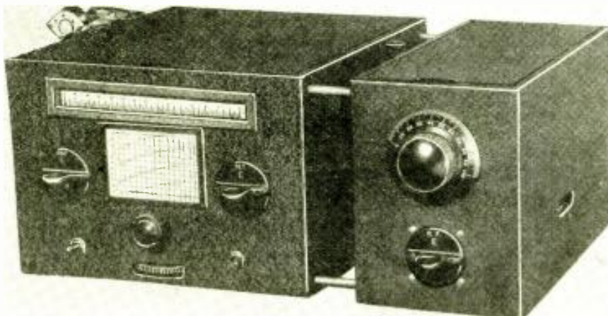
Appearance (left) and diagram (above) of the new National TRF Pre-Selector, for use ahead of the FB7 or other Super-hets (No. 148.)
